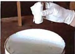
**Use gloves** enclosed and remove Syntho-Glass® from foil pouch.
